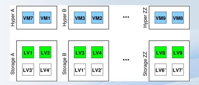
Any /dev/mars/\$vmname can appear at any machine whether "storage" machine or "hypervisor" machine *automatic* introduction of iSCSI-like network connections on port 7776 *backwards* compatible to classical MARS
